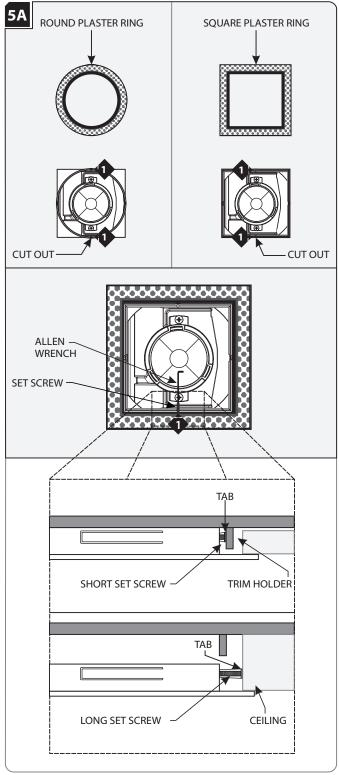
Insert the plaster ring completely into the collar/ceiling and secure them in place with the provided set screws and Allen wrench.
