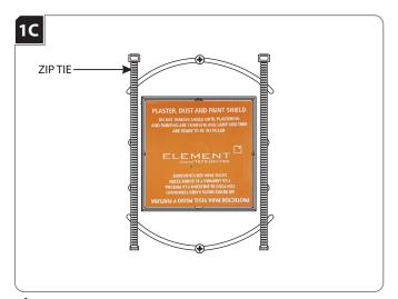
5 Carefully cut and remove the zip ties.
