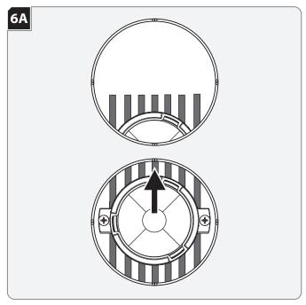
During shipping, the LED module and heat sink may shift on their track. Slide the module and heat sink into the center of the aperture until they lock into position.
